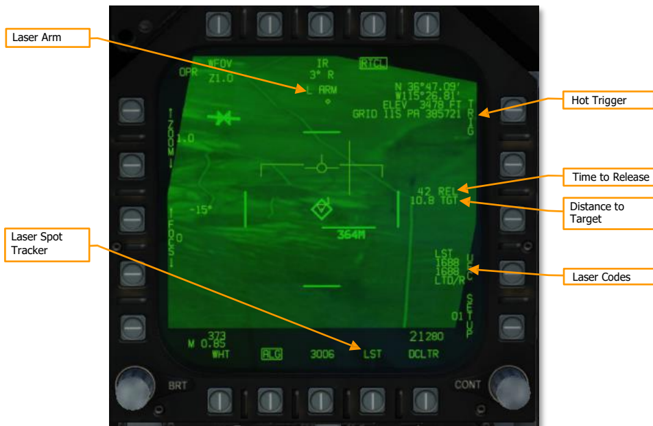
Figure 109. ATFLIR LTD/R and LST controls.
