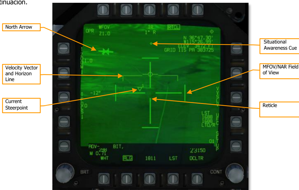
Figure 107. ATFLIR format in OPR mode (display elements).
